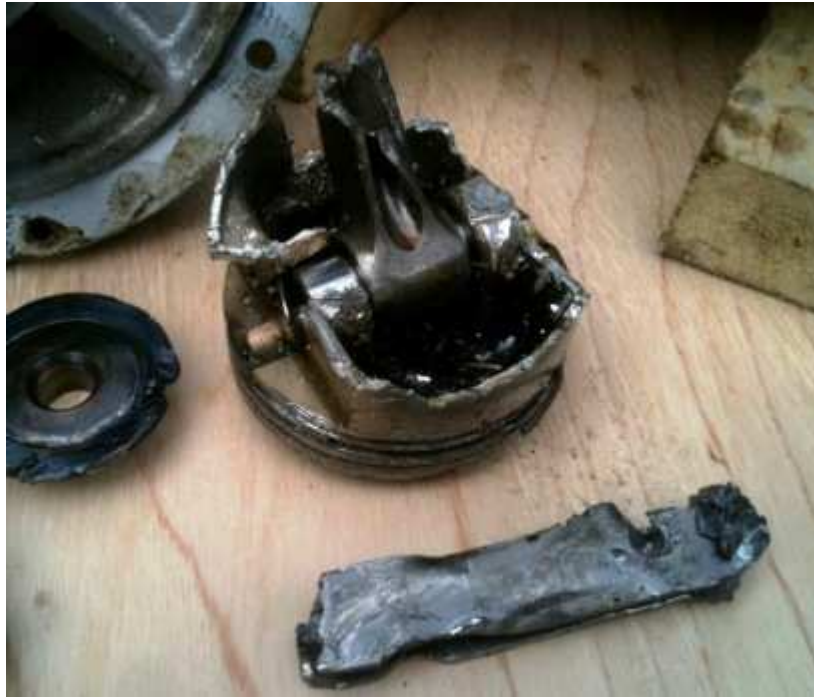
The remains of the piston and connecting rod
